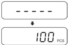
Remove reference weight. The balance is from now in parts counting mode counting all units on the weighing plate.
